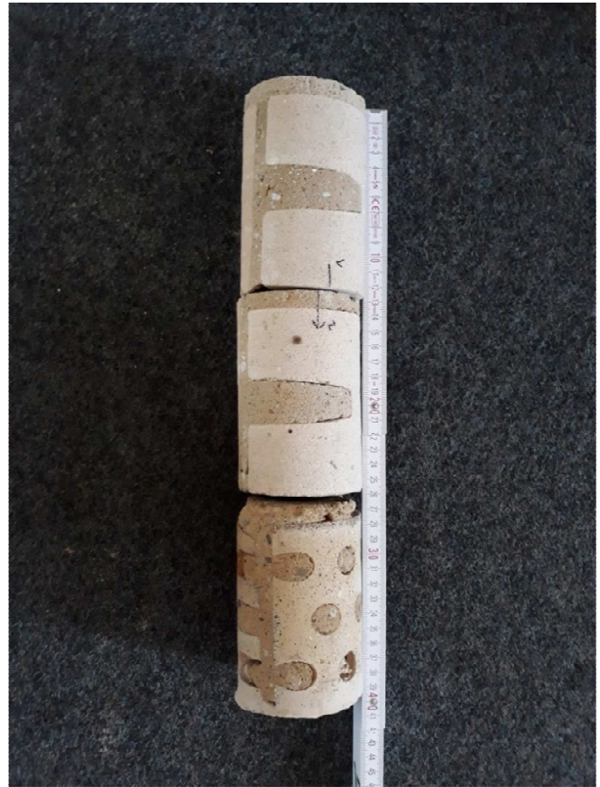
Bohrkern Wand West
